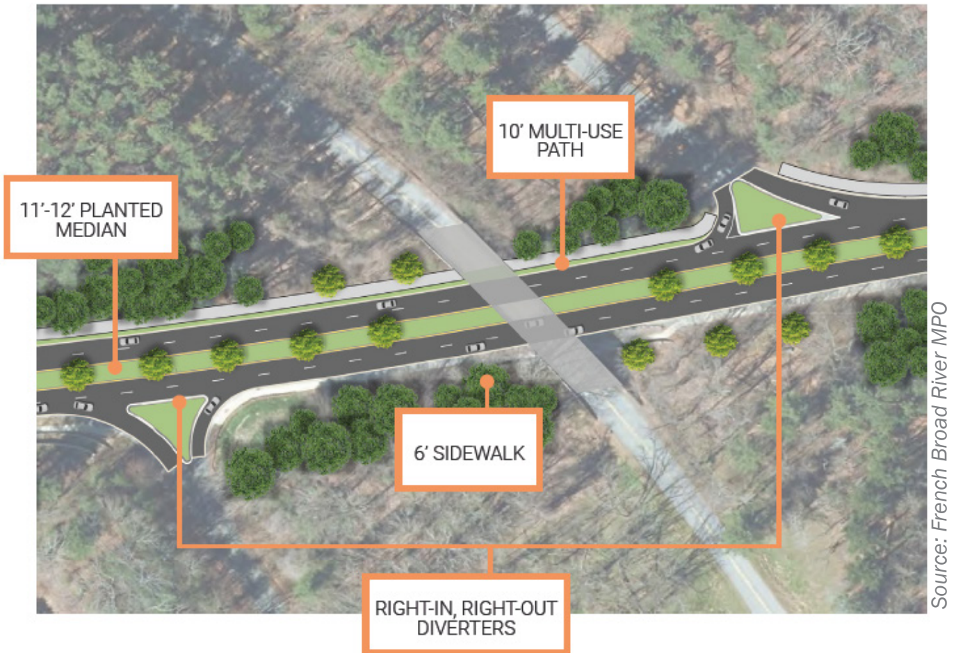
FIGURE 12 - BLUE RIDGE PARKWAY RAMPS (HENDERSONVILLE ROAD)
