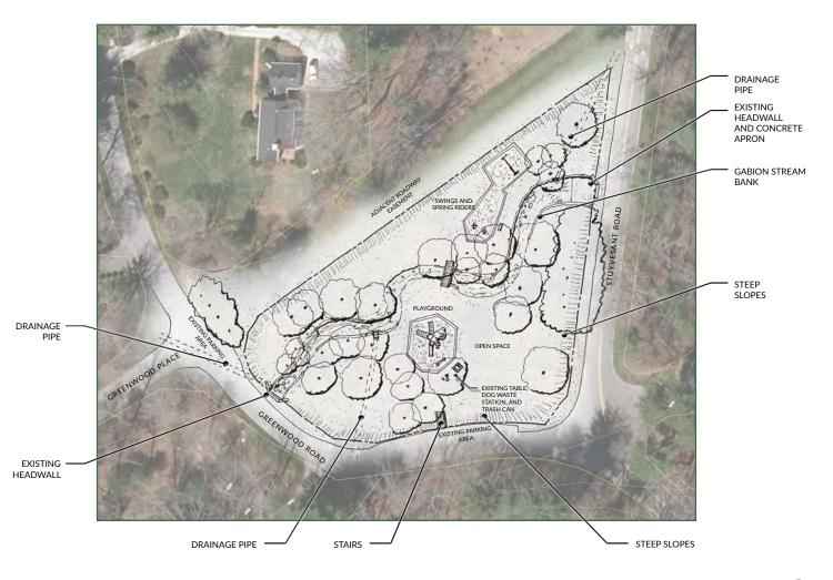
Portions of the stream have been stabilized with gabion walls, however these are beginning to fail and there is evidence of significant erosion beneath the gabion walls. The stream bed consists of a mix of rocks, sand, and vegetation, and can be easily accessed from the grass banks throughout the park.
