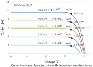
Current-voltage characteristics with dependence on irradiance and module temperature
